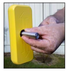
The CWT Detection standard is used to confirm that the T-Wand is functioning properly.
