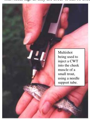
CWT, but cannot be used for half-length tags. A Wand Detector or V Detector are generally used alongside the Multishot to check each animal for the presence of a tag for quality control. The injector may be fitted with an electronic cycle counter as an option.
